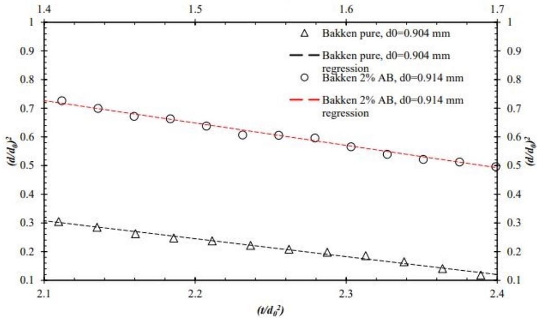
Figure 2.4 Zone IV comparison between Bakken crude and Bakken crude at 2%AB particle loadings
