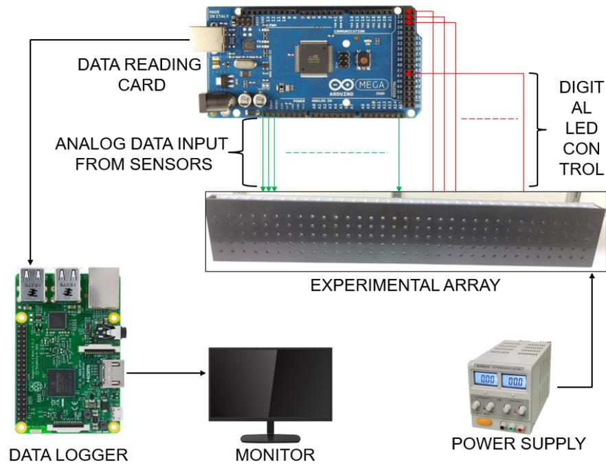
**Figure 2.13** Experimental layout for suspension stability analysis
