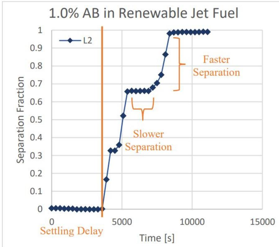
**Figure 2.15** Metastable state in 1% (w/w) AB suspension
