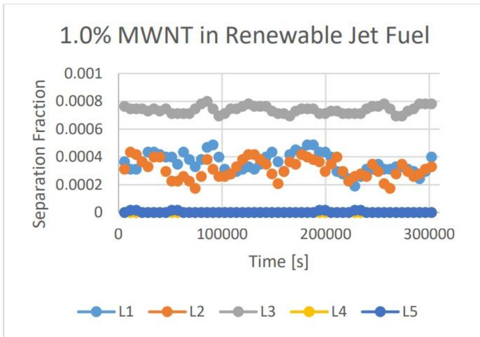
**Figure 2.17** Separation characteristics of 1% MWNT suspension
