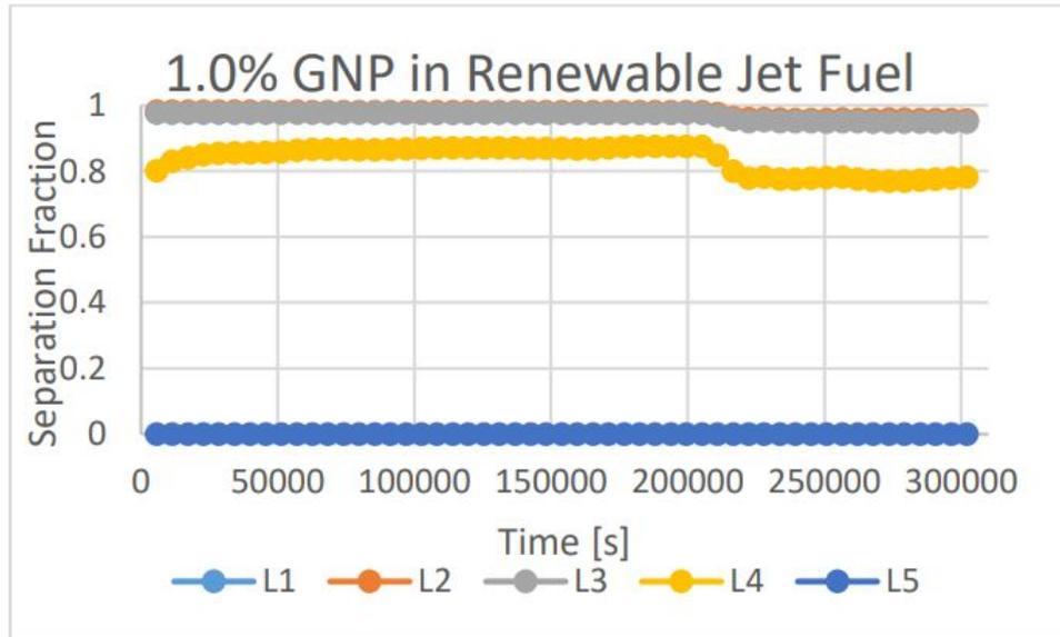
**Figure 2.18** Separation characteristics of 1% GNP suspension
